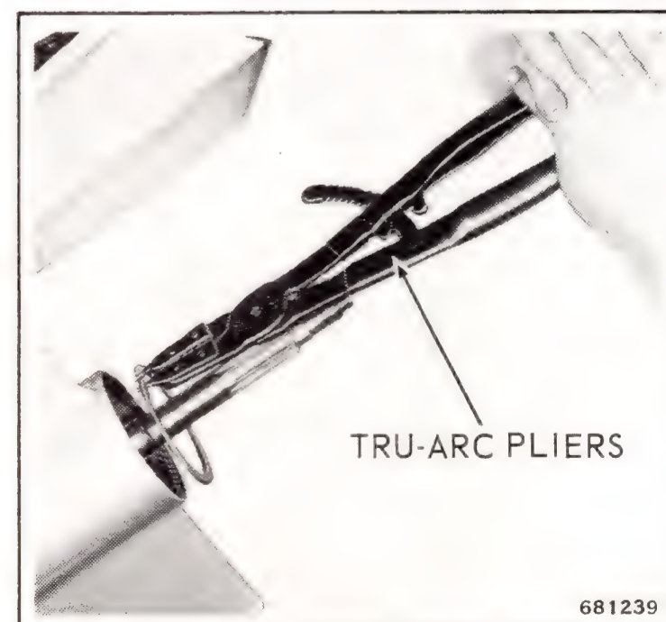
Figure 6-22. Remove Two Truarc Rings
