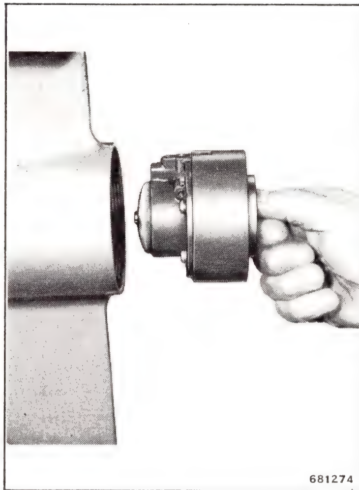
Figure 6-25. Removing Oil Pump
