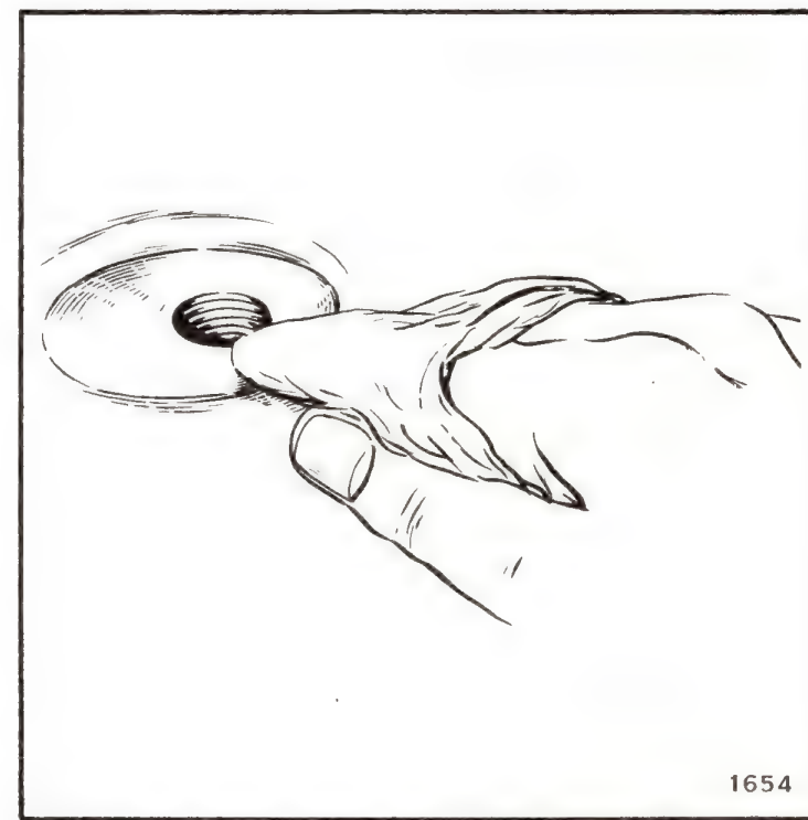
Figure 4-16. Cleaning Spark Plug Seat
