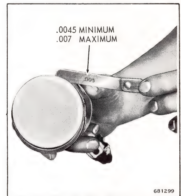
Figure 5-28. Checking Groove Side Clearance
