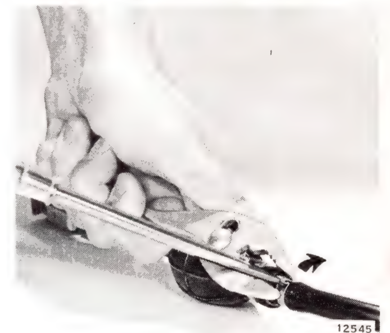
Figure 3-26. Removing Hose Clamps
