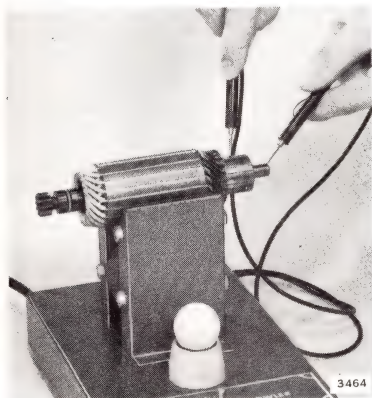
Figure 7-8. Checking Armature for Grounding
