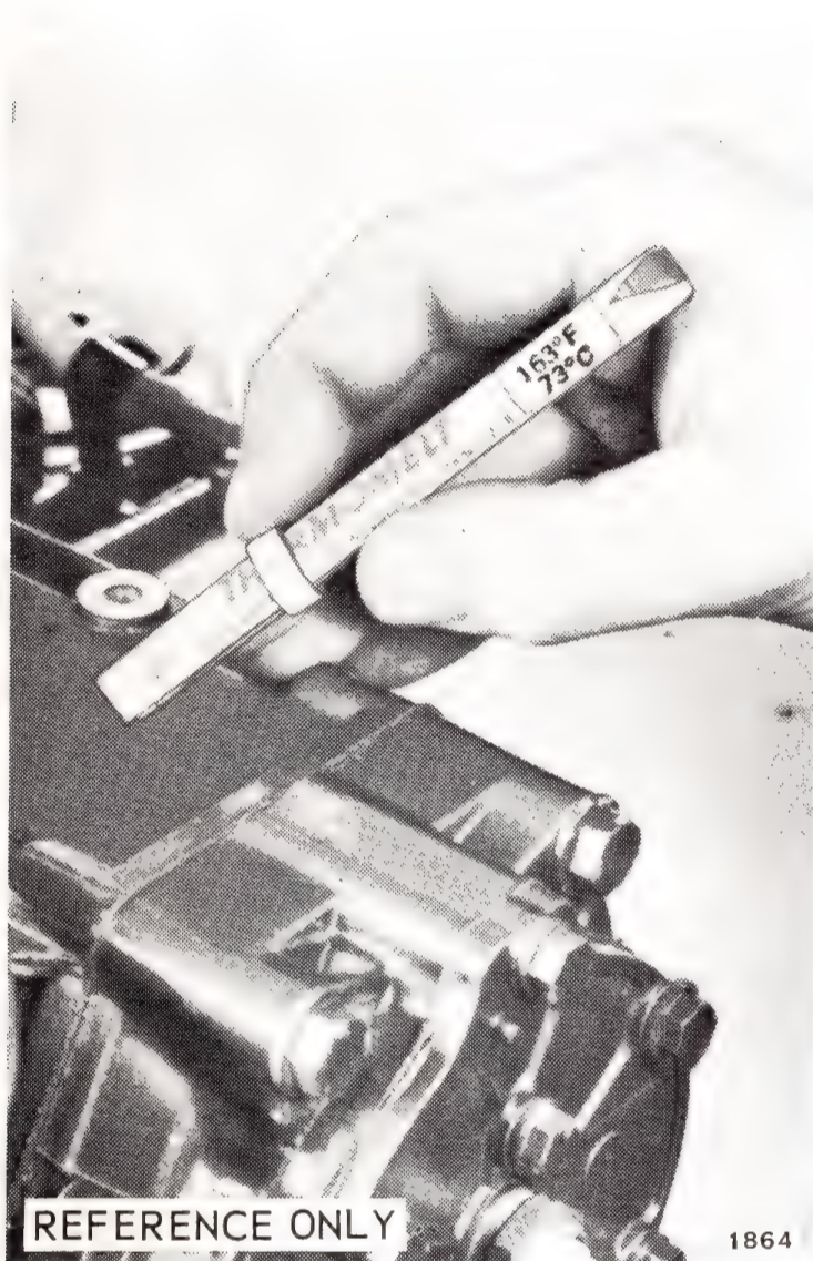
Figure 5-8. Checking Motor Temperature
